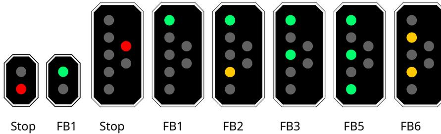
There are signal screens with 2, 3, 4 or 5 lights and double-width screens with a maximum of 7 lights; the 7th light is emergency
