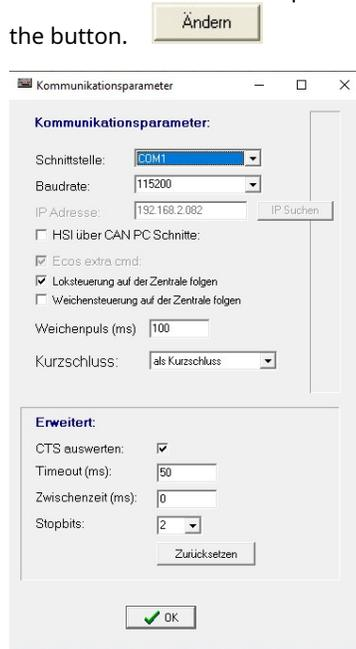
The interface used on the PC (COM1 - COM8, USB, ...) to which the control panel is connected must be specified here; only the existing interfaces are available for selection. If as an interface no is selected, no commands are sent from the PC to the digital center. In this way, the model signal box can also be tested or configured on a second PC without a model railroad connection.
