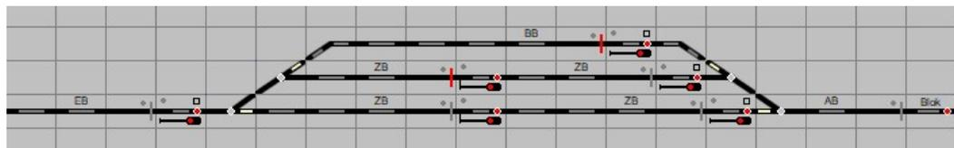
EB - entry block, BB - station block, ZB - central block, AB - exit block
