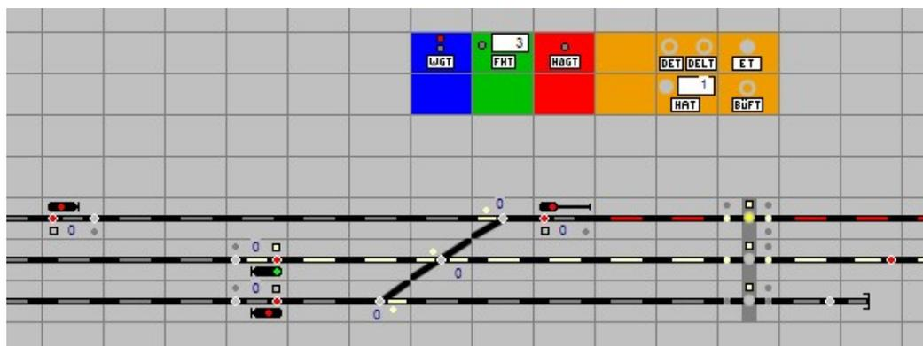
If a level crossing has more than one track, a separate level crossing is created as a solenoid for each track. This allows the level crossing to be closed and opened separately for each track with a route or with detectors. The level crossings are linked when defining the solenoid accessory. The solenoid article numbers of the other level crossings in the parallel tracks are specified in the input fields "BÜ in track above" and "BÜ in track below".
