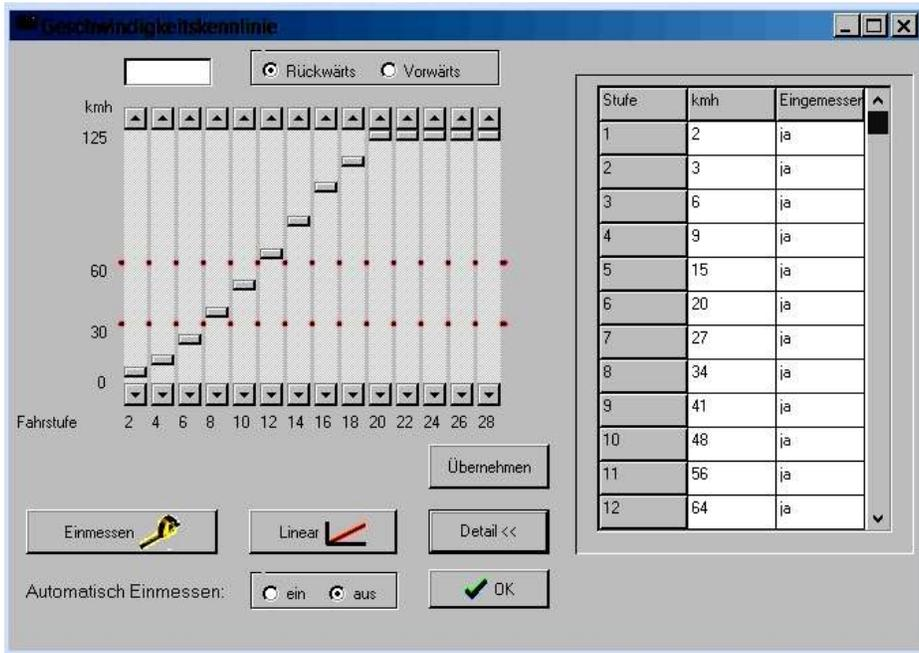
You can also edit the characteristics in table form with the [Detail] key.
