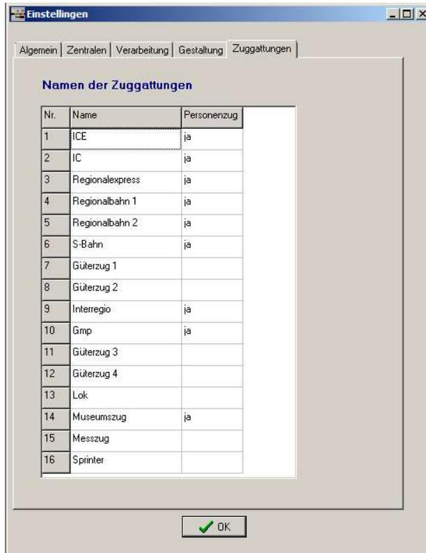
In this window you can change the names of the train types. For each type of train it is indicated whether it is a passenger train. This information is used for automatic braking (see Chapter 6.4.4.6).
