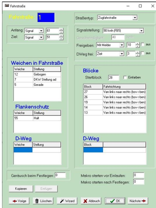
The window in which the data is entered consists of two parts. In the upper part the general data such as start and finish signal or destination button, type of route etc. are entered. In the lower part, the turnouts of the route are configured on the left and the blocks on the right. A route exists if the start and destination are entered.
