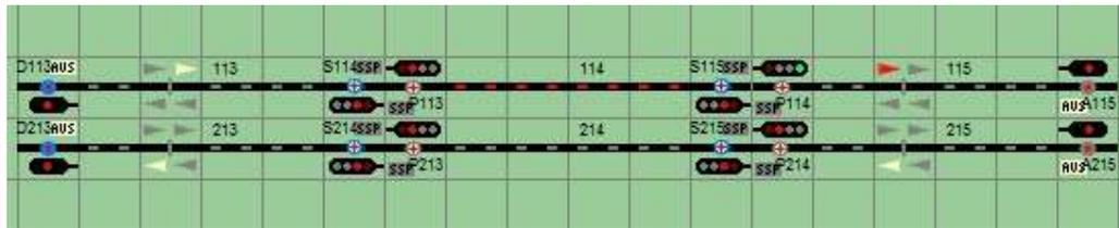
Example: 2-track line with a central block - the train is in section 114 - kilometrage
