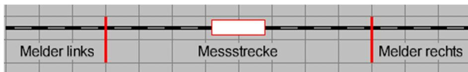
The measuring section has 3 sections / feedback contacts. The speed measurement is started with the locomotive on the measuring section; the measurement runs until one of the other contacts switches, depending on the direction of travel. The specified length is the distance between switching on and off. Make sure there is sufficient discharge on both sides of the measuring section.
