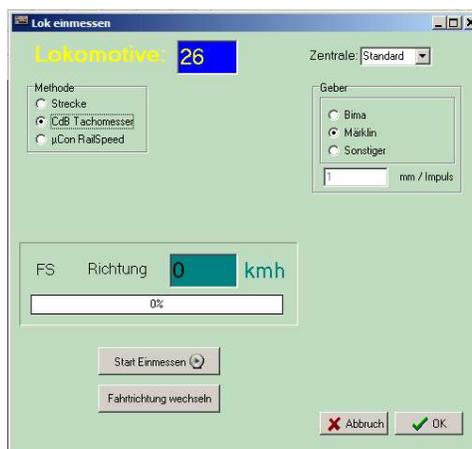
The selection "CdB speedometer" shows the input fields for calibration with the speedometer from CAN Digital Bahn.
