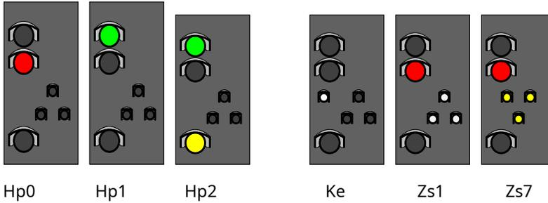
Block signal DB - block signals correspond to the main signals but cannot indicate the term Hp2. The signal aspects of a main signal are Hp0, Hp1, (Zs1, Zs7)
