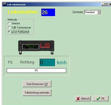
For calibration with the RailSpeed, a µCon Master must first be set up as the central unit (under Settings). This center is then selected in this window under "Central". It is not necessary to enter the address of the Railspeed, the calibration can take place at any Railspeed on the layout.
