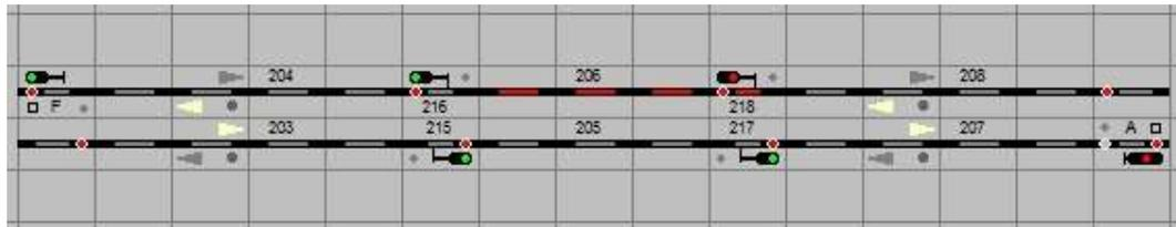
Numbering of the tracks and signals of a double-track block section - kilometering:
