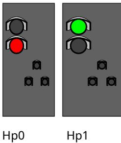
Main / blocking signal DB - possible signal positions: Hp00, Hp1, Hp2, Hp0 / Sh1, (Ke, Zs1, Zs7)
